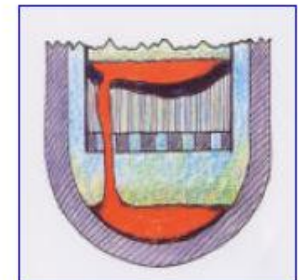
d) Corium relocation in the bottom vessel
