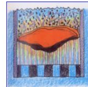
c) Crust, melt and debris bed formation
